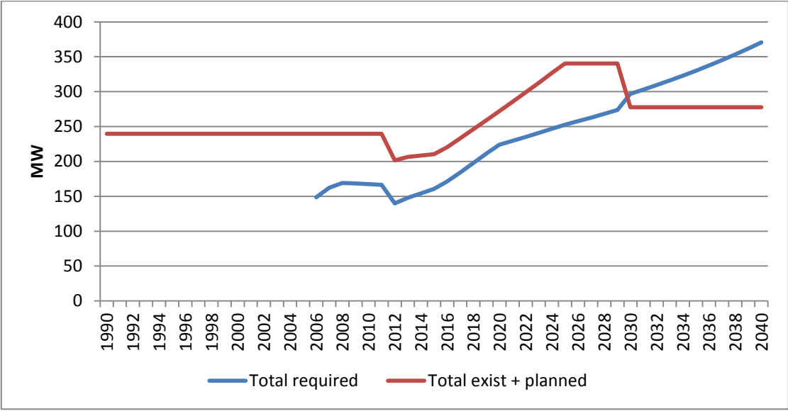
Figure 40: Electricity Demand Verses Supply under the Barbados Growth and Development Strategy Scenario
